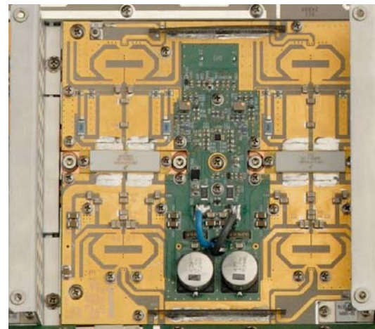
Figure 6 – 50V UHF LDMOS RF pallet
